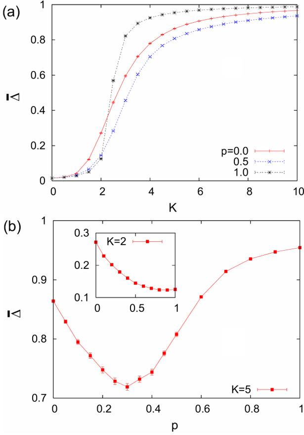
Fig. 2. (Color online) (a)  $\bar{\Delta}$  versus  $K$  at  $p = 0.0, 0.5$  and  $1.0$  for the network with  $L = 8$  and  $b = 3$  ( $N = 3280$ ). (b)  $\bar{\Delta}$  versus  $p$  at  $K = 5$ .  $\bar{\Delta}$  becomes smaller and then increases as  $p$  is increased. Inset:  $\bar{\Delta}$  versus  $p$  at  $K = 2$ . In contrast to  $K = 5$ ,  $\bar{\Delta}$  is observed to decrease as  $p$  is increased.
