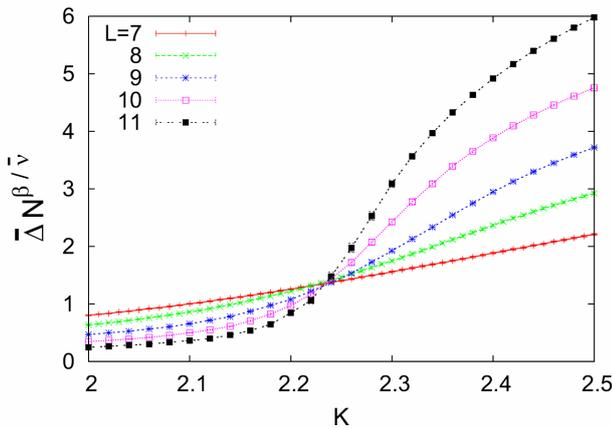
Fig. 4. (Color online) Scaling plot for  $\bar{\Delta} N^{\beta/\bar{\nu}}$  vs  $K$  at  $p = 1.0$  for  $b = 3$ . When  $\beta/\bar{\nu} = 0.2$ , which is the mean field value, crossing occurs at  $K \approx 2.23$ .
